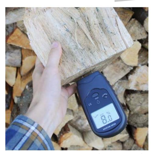
Burning wood which has less than 25% moisture content is more efficient and reduces the smoke from your chimney. A moisture meter can be a good way to check if your wood is ready to burn. Meters can be purchased for a relatively low cost or a limited number are available to borrow from the Invercargill Environment Centre.
