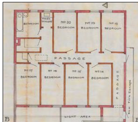
Figure 6-108. Detail of 1908 renovation plans showing first floor extension with rooms numbered 14 to 20 (ICC Property File).
