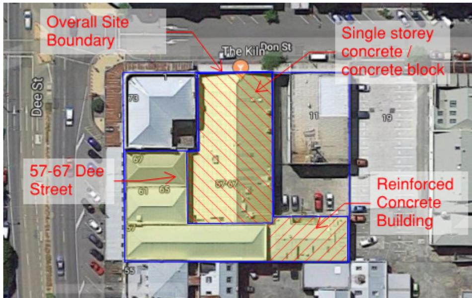
These conglomeration of buildings are in varying condition with the reinforced concrete and concrete block building sections appearing to be in relatively good condition.
