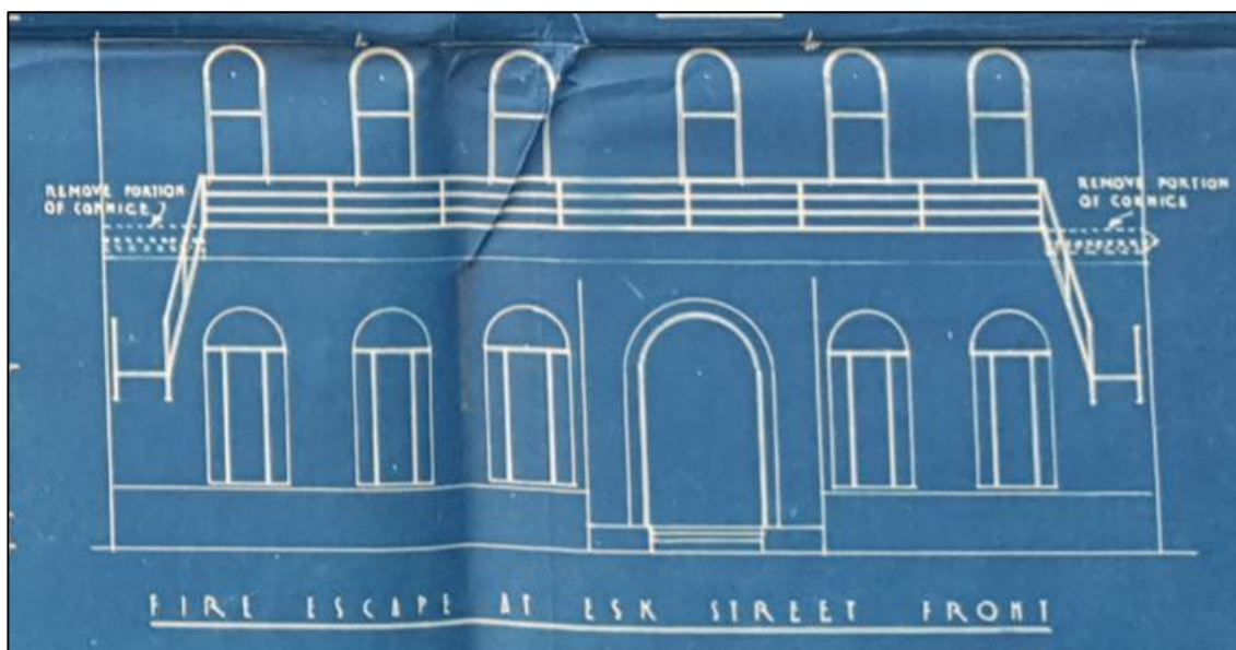
Figure 6-207. Detail from 1950 plan showing previous façade configuration (Ford, Gray, & Derby, 1950).
