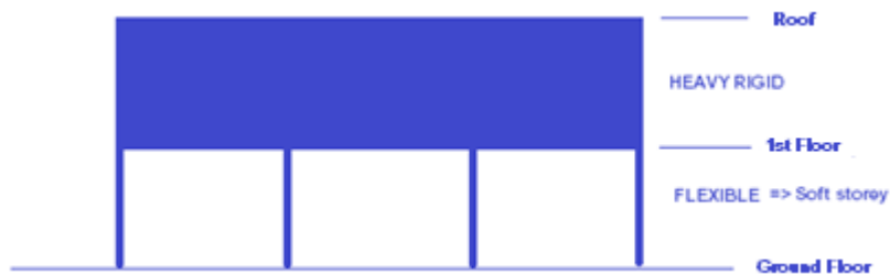
Figure 3 - Building elevation of soft storey structure example
