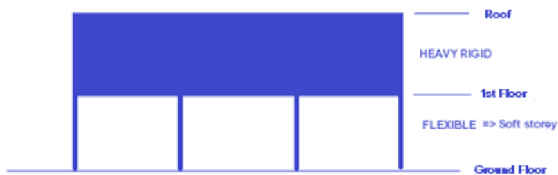
Figure 3 - Building elevation of soft storey structure example
