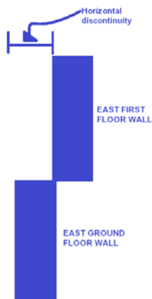
Figure 3 - Horizontal discontinuity along east elevation of building
