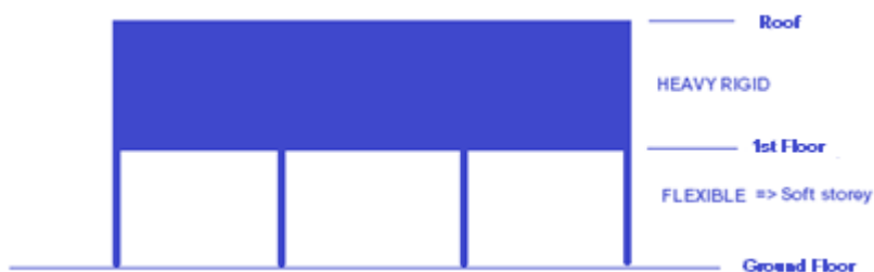
Figure 4 - Building elevation of soft storey structure example
