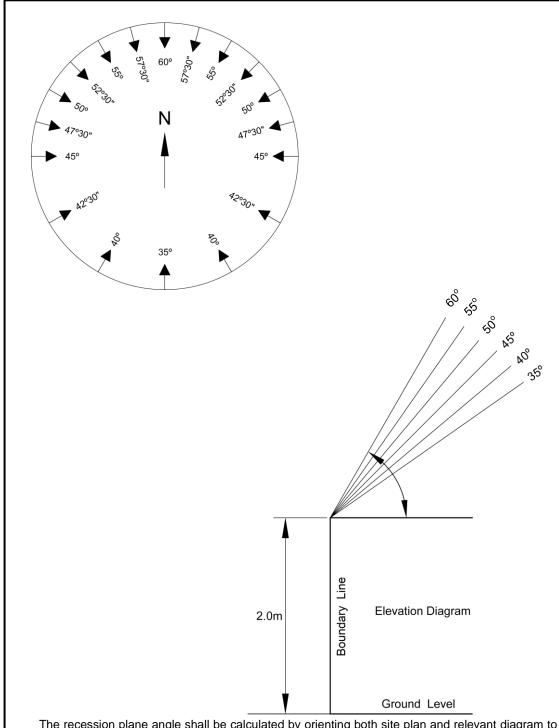
The recession plane angle shall be calculated by orienting both site plan and relevant diagram to the true north, placing the recession diagram over the site plan with the circle tangential to the inside of the site boundary under consideration. The recession plane angle shall be that indicated by the diagram at the point where it touches the site boundary. Where recession lines fall between those indicated on the diagram, interpolations shall be made.
