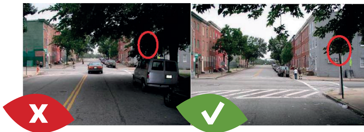
Figure 18 : Left shows the incorrect way and right shows the correct location of the tree relative to the street light so as not to obstruct it.
