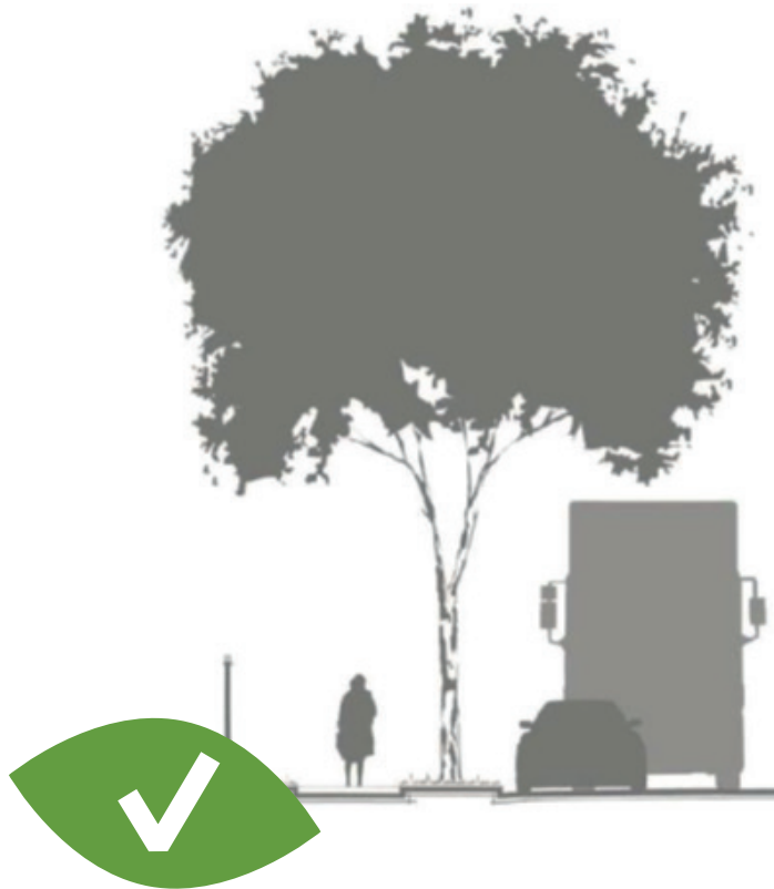
Figure 5: Large trees progressively pruned to clear footpath and a carriageway but natural attractive crown form preserved. Crown should be clear of bin arm with a 4m height clearance.
