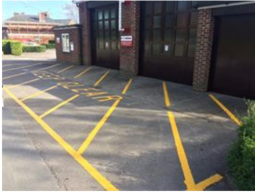
Figure 6-1 : Example of Keep Clear hatching
