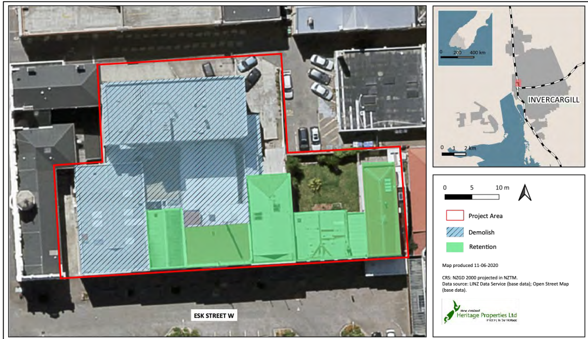
Figure 8-1. Flexible option for retention versus demolition - allows a larger individual footprint in a new build if required.
