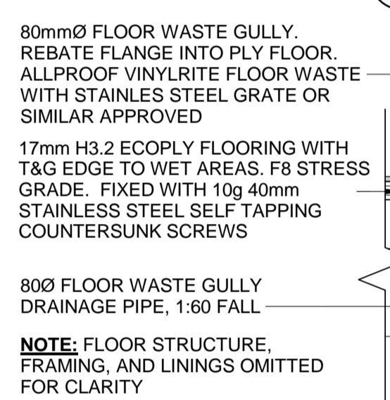
9 FLOOR WASTE GULLY A400 1:5
