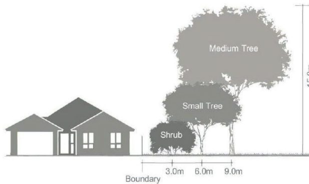
Figure 1: Reserve planting setback distances from private property boundaries in relation to potential tree size
