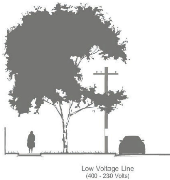
Figure 9: Large growing tree in maturity planted to side of power lines, showing pruning method to clear lines.
