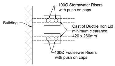
Note: this detail is for a 150mm dia property connection, where the property connection is 100mm dia reducing wye junctions are not required.
