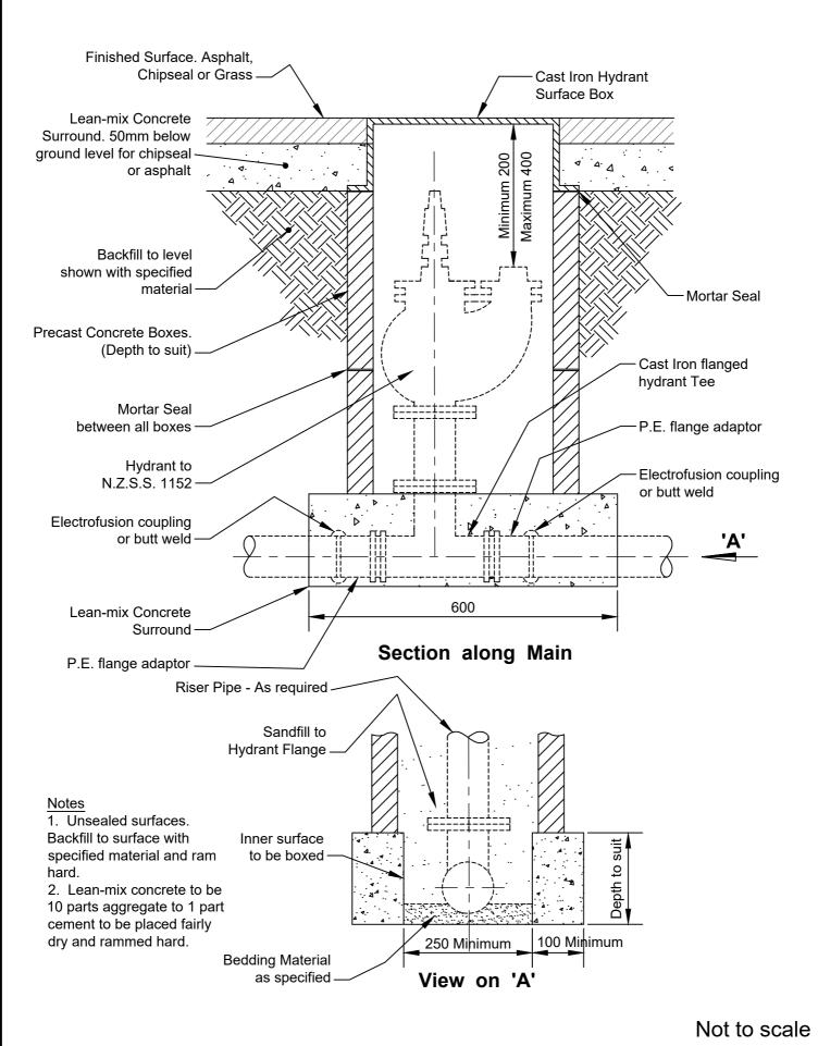
HYDRANT INSTALLATION WITH FLANGE ADAPTOR
